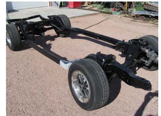
All frames are sand blasted and Powder-coated to better than factory luster
